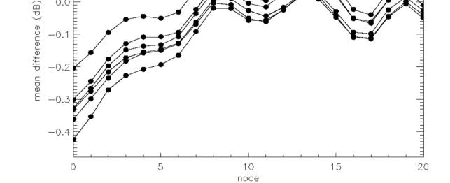
Oscillations in the difference between sea ice backscatter and ice line model in the left fore beam, 2007-2013
