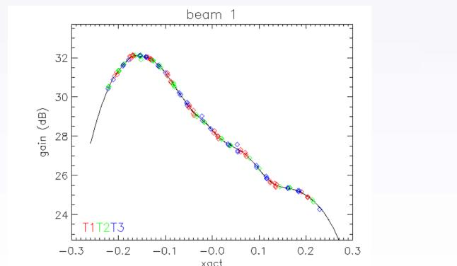
Set of transponder data with fitted gain model
